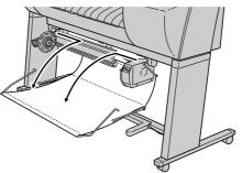
Store the output stacker where it will not interfere with the sensors.
